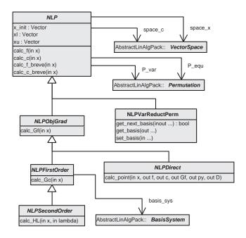
Figure 3. UML class diagram: NLPInterfacePack, abstract interfaces nonlinear programs
