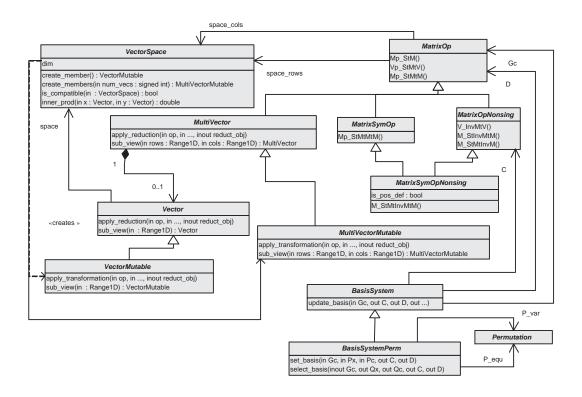
Figure 2. UML class diagram : AbstractLinAlgPack, abstract interfaces to linear algebra
